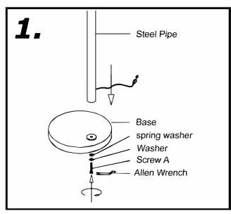
Screw the **Steel Pipe** onto the **Base** with **Screw A, Spring Washer**, and **Washer**. Then, tighten up with the provided **Allen Wrench**.
