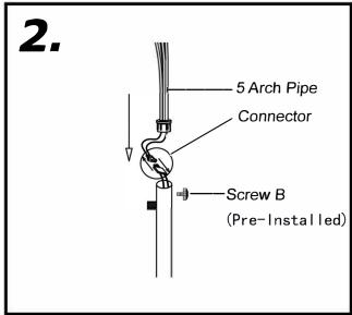
Link up the Male and female **Connector** together. Insert the **5 Arch Pipe** into the **Steel Pipe** and Secure it with the **Screw B**.
