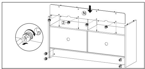
**Step13**: Bring the product to upright position. Insert Back Board (N) as figure. Insert Camlock (HW2) then tighten using screwdriver as figure.
