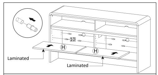
**STEP15**: Insert Shelf Pin (HW10) into the holes on Center Boards and Side Boards, on the desired level. Then place the Adjustable Shelf (H) by inserting the grooved line on the shelf into the shelf support, with laminated edge facing front.
