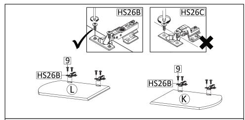
**STEP16**: Insert Hinge (HW HS26B) into 1 piece of Door Left (K) and 1 piece of Door Right (L). Secure with Screw M4.5x12.5mm (HW9).
