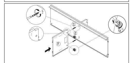
**Step7**: Insert Cambolt (HW1) to Fixed Shelf (E). Attach Center Board 1 (F) as figure. Secure with Camlock (HW2) then tighten using screwdriver.
