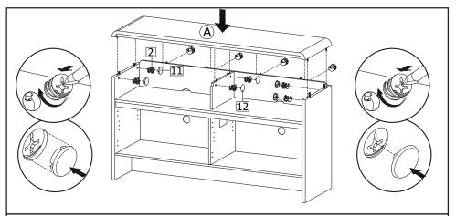
$\bf STEP14: Attach\ Top\ Board\ (A)\ into\ Body\ .$  Insert Camlock (HW2) then tighten using screwdriver. Put Screw Caps (HW11&HW12) over the camlock as picture.
