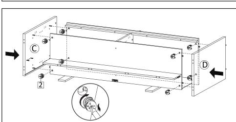
**STEP11**: Attach Side Board Left (C) and Side Board Right (D) into Bottom Board (B) and Fixed Shelf (E). Insert Camlock (HW2) then tighten using screwdriver.
