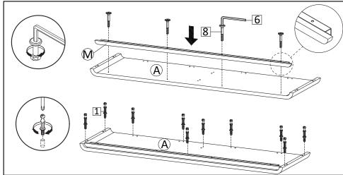
**STEP4**: Insert Screw M6.4x35mm (HW8) into Front Skirt 2 (M) into Top Board (A) tighten screws using Allen Key (HW6) as figure. Insert Cambolt (HW1) into Top Board (A).
