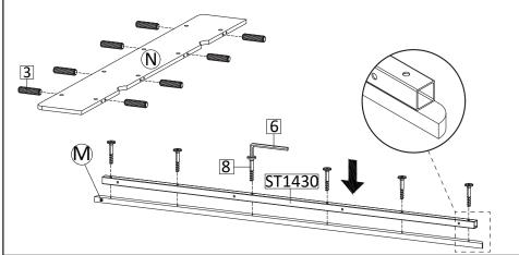
STEP3: Insert Dowel Small (HW3) into Back Board 1 (N). Attach Anti Deflection Bar (HW ST1430) into Front Skirt 2 (M) using Screw M6x35mm (HW8) then tighten using Allen Key (HW6) as figure.
