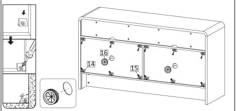
**STEP20**: Use Wedge (HW14), Screw M3.5x15.5mm (HW15) to tighten the back of Sideboard by using screwdriver. Please align the top board and bottom board in  $90^{\circ}$  position against the side board, before securing the wedges (HW14). Insert Cable Hole Rubber (HW16) as figure.
