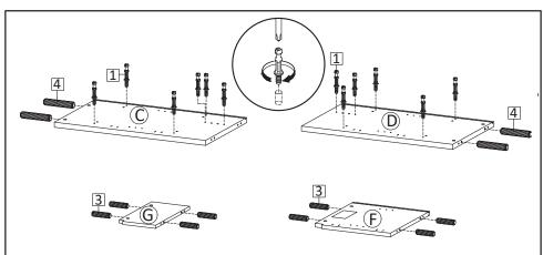
**STEP1**: Insert Cambolt (HW1) and Dowel Big (HW4) into Side Board Left (C) and Side Board Right (D). Insert Dowel Small (HW3), Center Boards 1 (F) and Center Board 2 (G) as figure.
