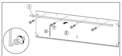
**STEP5**: Attach Front Skirt 1 (I) to Fixed Shelf (E), secure with Screw M6.4x53mm (HW7). Tighten screws using Allen Key (HW6).
