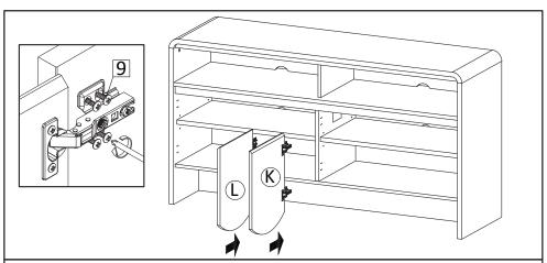
**STEP17**: Install Door Left (K) and Door Right (L) into Center Boards Please review above images carefully. Secure with Screw M4.5x12.5mm (HW9). Refer to separate page of how to adjust hinge (HS26B).
