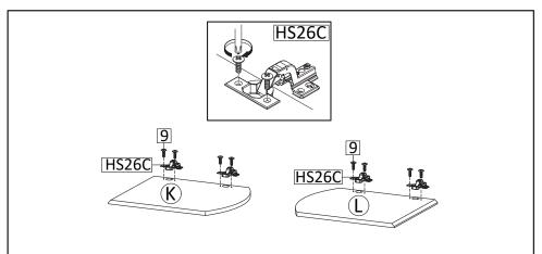
**STEP18**: Insert Hinge (HW HS26C) into remaining Door Left (K) and Door Right (L). Secure with Screw M4.5x12.5mm (HW9).
