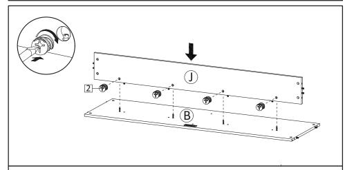
**Step8**: Attach Bottom Skirt (J) into Bottom Board (B). Insert Camlock (HW2) then tighten using screwdriver.
