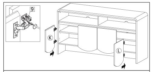
**STEP19**: Install Door Left (K) and Door Right (L) into Side Boards Please review above images carefully. Secure with Screw M4.5x12.5mm (HW9). Refer to separate page of how to adjust hinge (HS26C).
