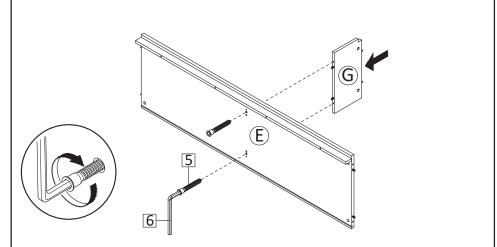
**Step6**: Attach Center Board 2 (G) to the Fixed Shelf (E). Secure with Screw M7x50mm (HW5), tighten screws using Allen Key (HW6).
