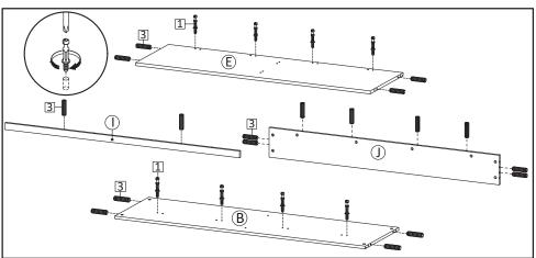
**STEP2**: Insert Cambolt (HW1) and Dowel Small (HW3) into Fixed Shelf (E) and Bottom Board (B). Insert Dowel Small (HW3) into Front Skirt 1 (I) and Bottom Skirt (J) as figure.
