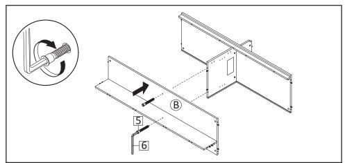
**Step9**: Combine Bottom Board (B) to assembled component from step 7 as figure. Insert Screw M7x50mm (HW5), tighten screws using Allen Key (HW6).
