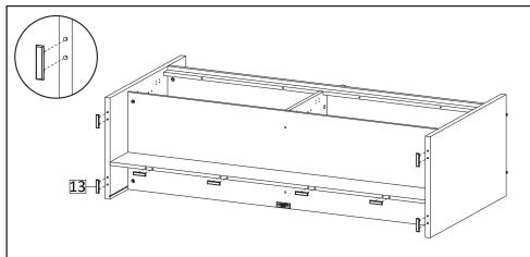
**Step12**: Insert Floor Glide (HW13) into Side Boards and Bottom Skirt as figure.
