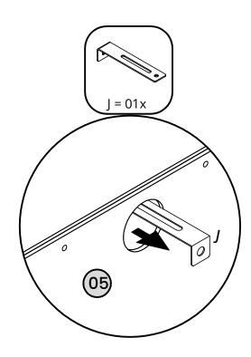
Then, pass the hardware ( J ) through the hole of the part (05) from inside to the outside as shown in the figure above until it reaches the wall.
