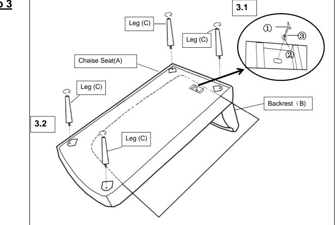
Step 3.1 Position the Chaise on its back, as shown. Attach the Chaise Back (B) to the Chaise Seat(A) using Horn screw (①), Washer (②), Spring Washer(③). Step 3.2 Install the Leg (C) into the Chaise Seat(A) and Chaise Back(B). Tighten the Leg by turning clockwise.
