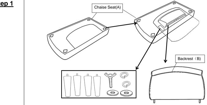
Position the Chaise Seat(A) facedown on a clean, non-marring surface. Unzip the pouches and remove the Backrest(B) and Legs(C) and Horn screw (1), Washer (2) and Spring Washer(3) from the bottom of the chaise, Zip-up the pouch.
