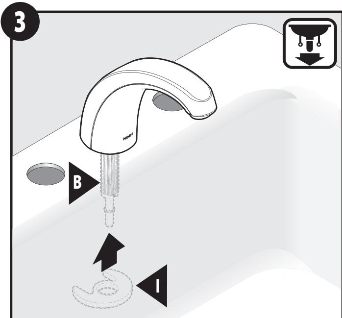
From below the deck, slide Mounting Bracket (I) onto Spout (B) shank.
