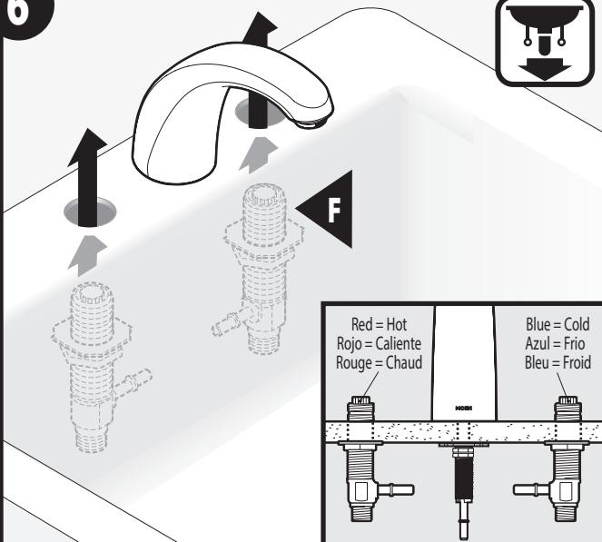
From below the deck, insert each Valve Body (**F**) into remaining sink holes. Ensure hot side valve body is on the left and the cold valve body on the right as shown. Hand tighten hardware to underside of deck.
