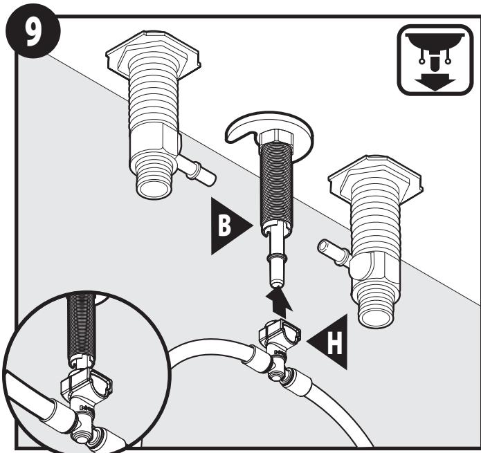
Install Quick Connect Hose (H) onto Faucet Body (B). Push up as far as possible until a click is heard. Tug downward to test engagement.
