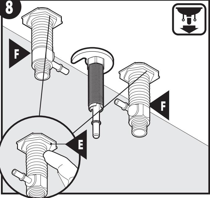
Ensure mounting hardware is snug and secured to underside of deck. Tighten until secure by hand.
