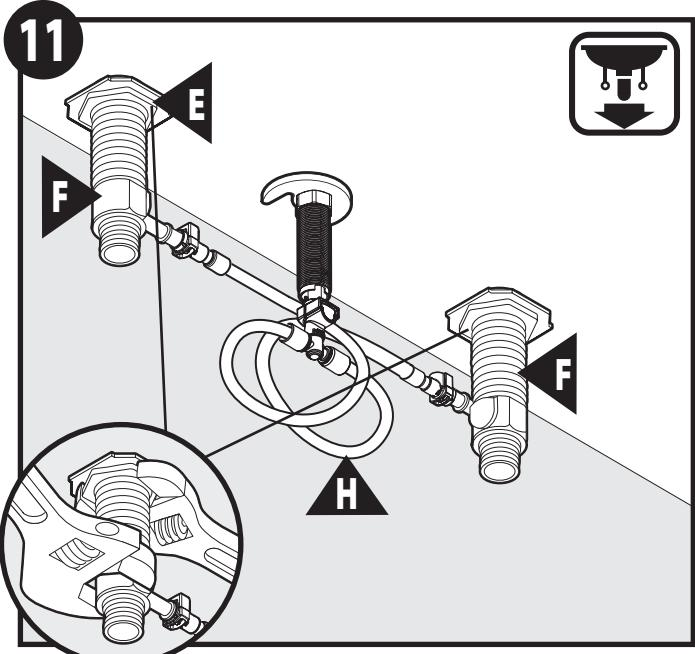
Once Quick Connect Hose (H) is secure, use adjustable wrenches to further tighten mounting hardware. Place one wrench on Valve Body (F) to hold in place while other wrench tightens Mounting Nut (E).
