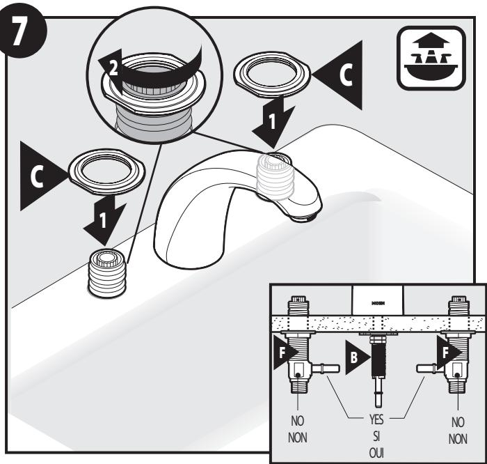
Install each Top Mounting Nut (**C**) onto each Valve Body (**F**) by threading downward onto sink. Ensure both Valve Bodies point towards Spout (B) shank.
