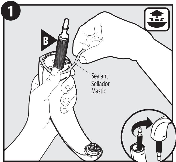
Apply a bead of plumber's sealant to underside of Spout (B). Flip over to place into sink.
