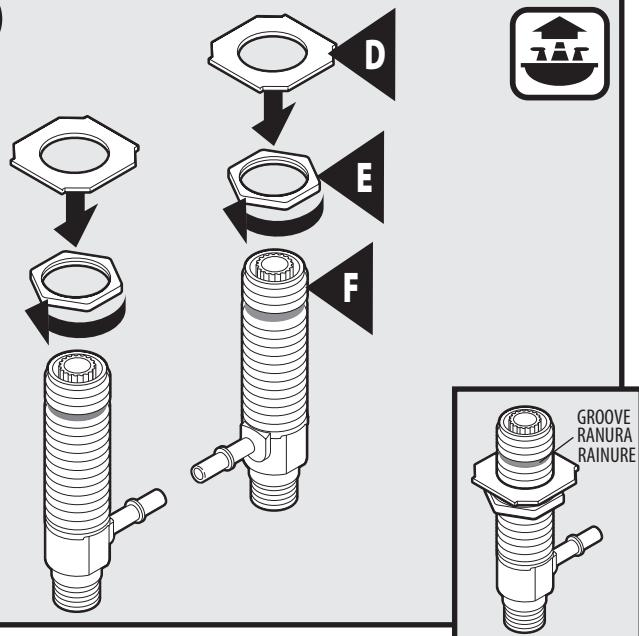
Assemble and thread the Valve Body Washer (**D**) and Valve Body Mounting Nut (**E**) onto each Valve Body (**F**) until they are resting below the valve body groove as shown.
