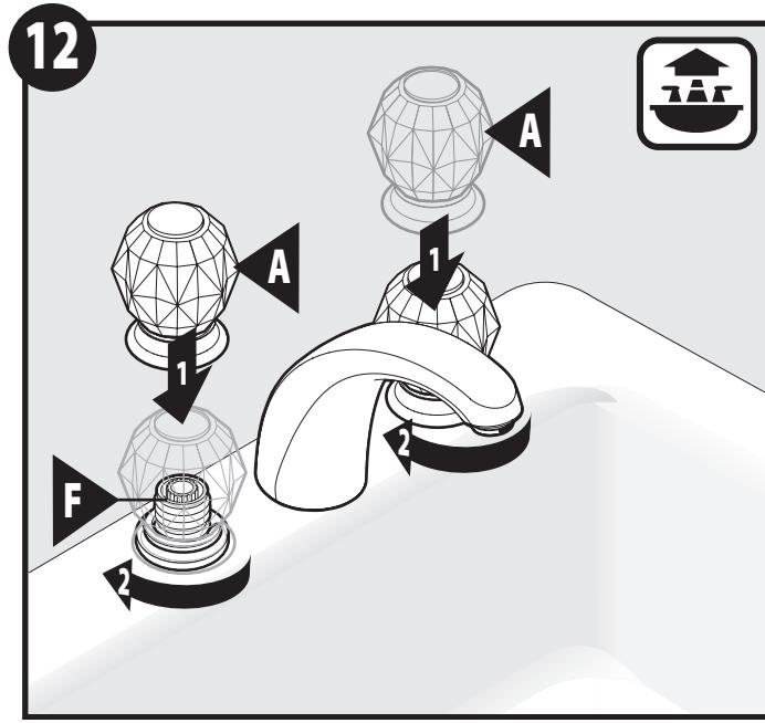
Install Handles (A) by threading onto each Valve Body (F). Secure to sink deck.
