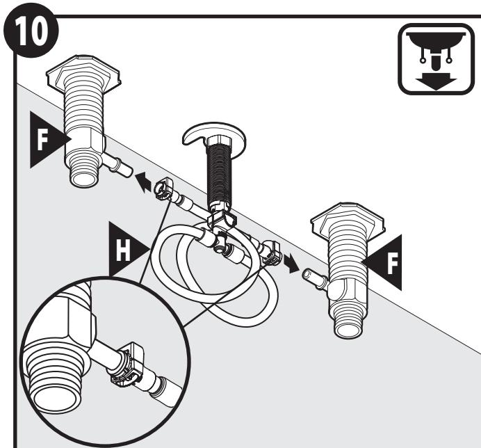
Install each end of Quick Connect Hose (H) onto Valve Body (F) as shown. Push each end as far as possible until a click is heard. Tug on each connection to test engagement.
