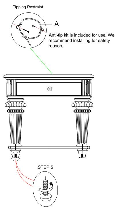
Adjust Leveler if needed to level case on uneven floor.
