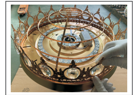
Step 7. Install the crystal into the fixed hole on the side of the lampshade.
