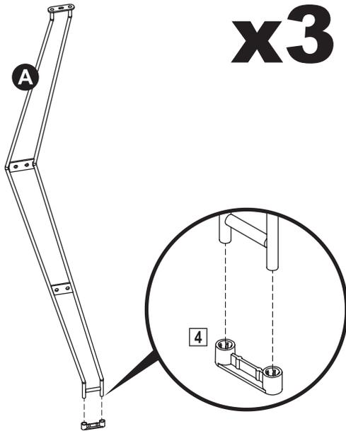
Firmly push one Plastic Foot (4) onto the bottom of Leg (A).
