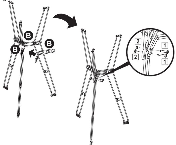
As indicated in the drawing, align three Upper Supports (B) with the top of Legs (A) and secure using six M6x25mm Screws (1) and six M6 Nuts (3).
