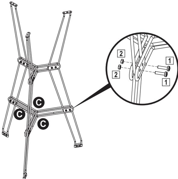
Align three Lower Supports (C) with the bottom of Legs (A) and secure using six M6x25mm Screws (1) and six M6 Nuts (3).
