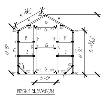
**Step 9:** Finally – measure your structure to determine the amount of materials you will need to purchase to cover your structure. Always make sure you allow for seams or waste material and purchase extra. To determine the amount of material needed for the front and rear of the structure measure the base for your width and then measure from the base to the top of the ridge for your height.
