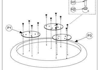
\*Screw the bolts out to take frame out (P1) of top (P3)
