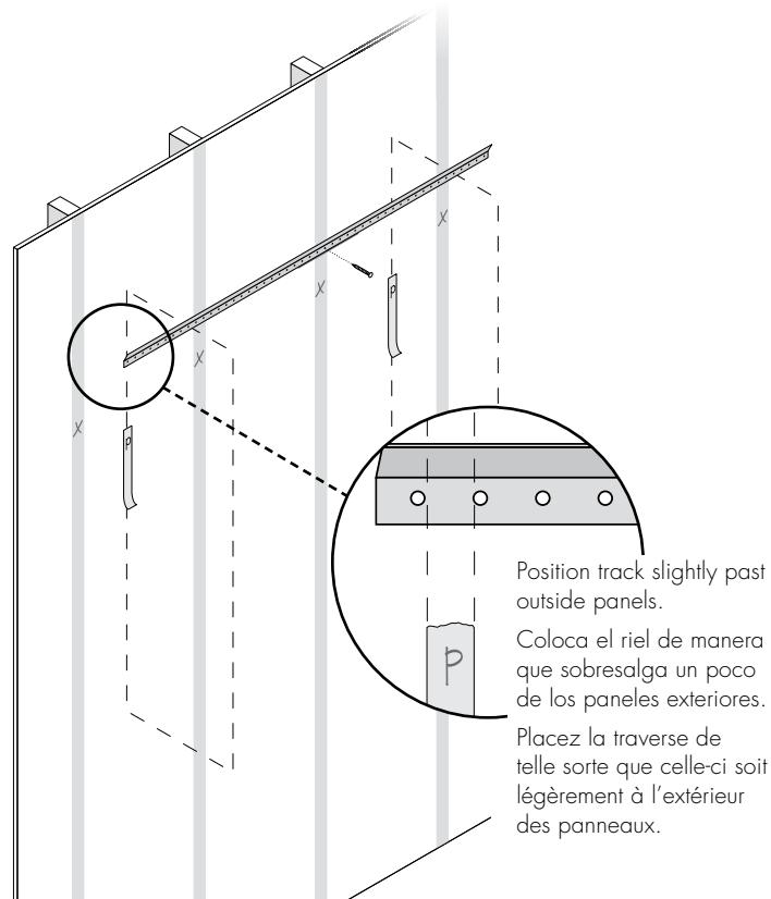
**5** Level the track and mark a line along its bottom edge. Drill  $\frac{1}{8}$ " pilot holes into each stud location and in the last hole of the track on both ends of the wall.
