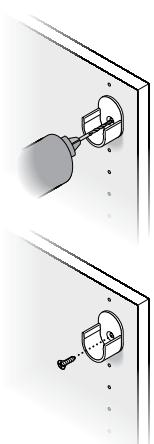
Drill  $\frac{1}{8}$ " pilot holes into vertical panels through the existing hole in rod holders.
