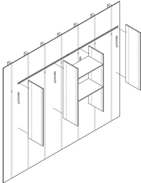
**13** Install rod holders on the vertical panels. Snap wardrobe rods into place. Install adjustable shelf with shelf pins.
