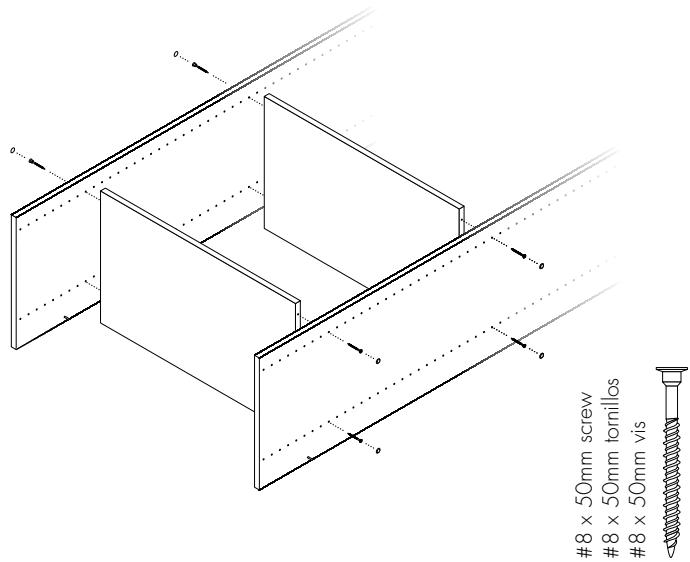
**12** Hang assembled center unit and shorter vertical panels in their marked positions.
