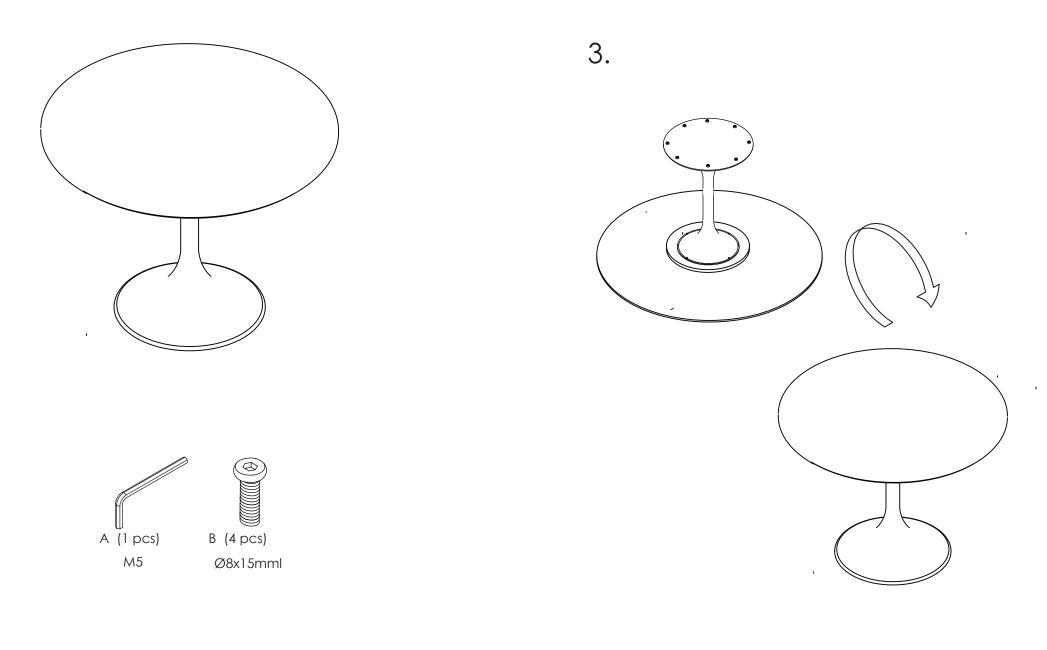
During assembly, hand tighten screws only. When the screws are in place, tighten completely.
