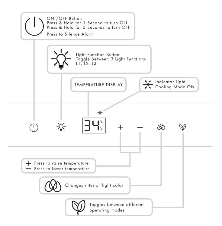
The temperature setting can be adjusted from 34-50°F. Your controls are simple and intuitive to operate.
