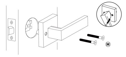
Attach the indoor handle lock to the square bolt on the outside and align the screws from the interior latch towards the posts. Tighten the screws and test the lock.
