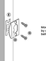
Mount the strike onto the door frame by aligning it with the latch height before drilling the required holes.
