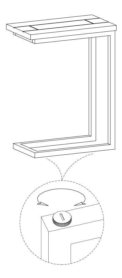
**Note**: Levelers on bottom of legs can be adjusted if floor is uneven.
