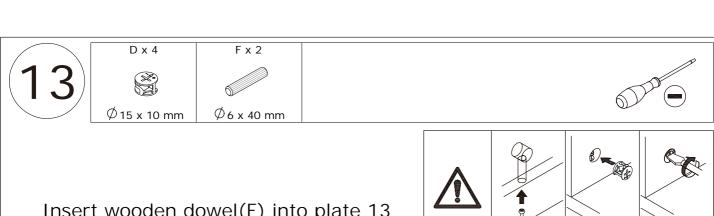
Insert wooden dowel(F) into plate 13 at first.
