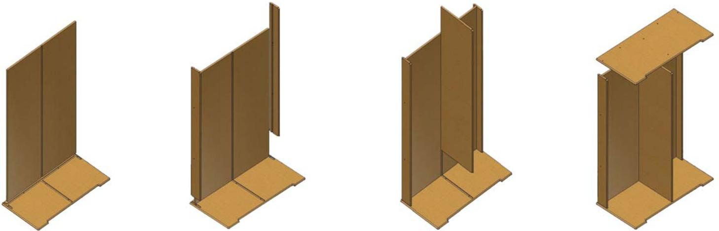
**Step 1:** Attach **Top** to **Side**, aligning groove in underside of Top with dado in Side. Attach components together with (2) Hex screws and Allen wrench.
