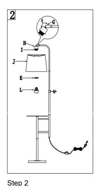
Put the shade(J) on the socket(I),then tighten the out ring(K) on it.
