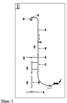
Make sure all parts could be aligned before assemble Unpack all parts from cartons carefully. Check and make sure all parts are present. Screw the Metal tube(B)onto the Lamp base(A) Screw the Metal frame(C)onto the Metal tube(B) Screw the Metal pallet(D)onto the Metal frame(C) Screw the Metal tube(E)onto the Metal frame(C)
