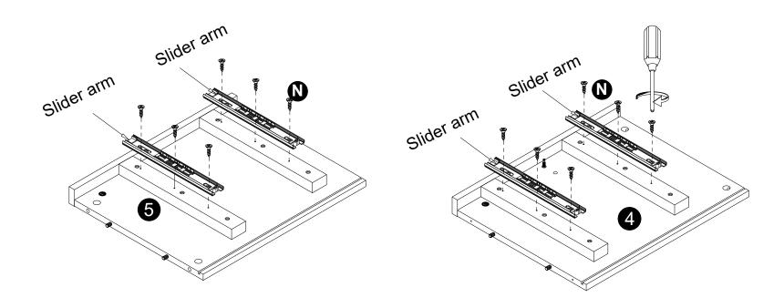
· Attach slider arms to panels (4,5) with screws (N) correctly.
