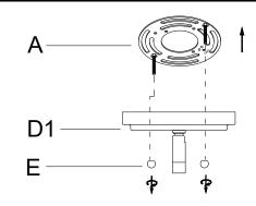
**Step 1:**Unpack all parts from cartons carefully. Separate the Mounting Plate(A) from the Canopy(D1) by removing the Canopy Nut(E) anti-clockwise.
