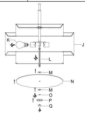
Step 7:Insert the bulbs(K) into the sockets until secure.DO NOT EXCEED THE SPECIFIED WATTAGE.Insert the Threaded tube (L) into the tube of the sockets assembly of Shade (J). Position 1 Plastic washer (M), then place the Diffuser (N) onto the threaed tube. Place another Plastic washer (M), fix it by turning the Hex Nut (O) clockwise till tight. Place the Metal Cover (P) through the theaded tube, fix the Metal Cover (P) in place by turning the Finial (Q) clockwise till tight.
