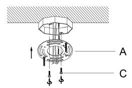
Step 3: Insert the Long tube(G) into the thread portion of the Swivel (D2) and the Canopy(D1), Step 4: Attach the Mounting Plate (A) to the ceiling junction box and secure it by tightening 2 Mounting Screws (C) with a screwdriver until secure.
