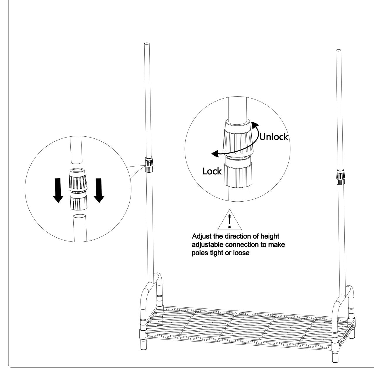
Connect the Hanger Rod(D)and hanger upper tubes by Corner Connectors(F).
