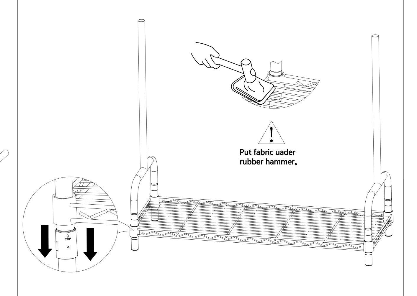
Insert Hanger Upper Tubes(C)into Y-shaped poles by Height Adjustable Connectors(E) to make them confirm. Make sure the height adjustable connectors in unlock status before connect two poles.
