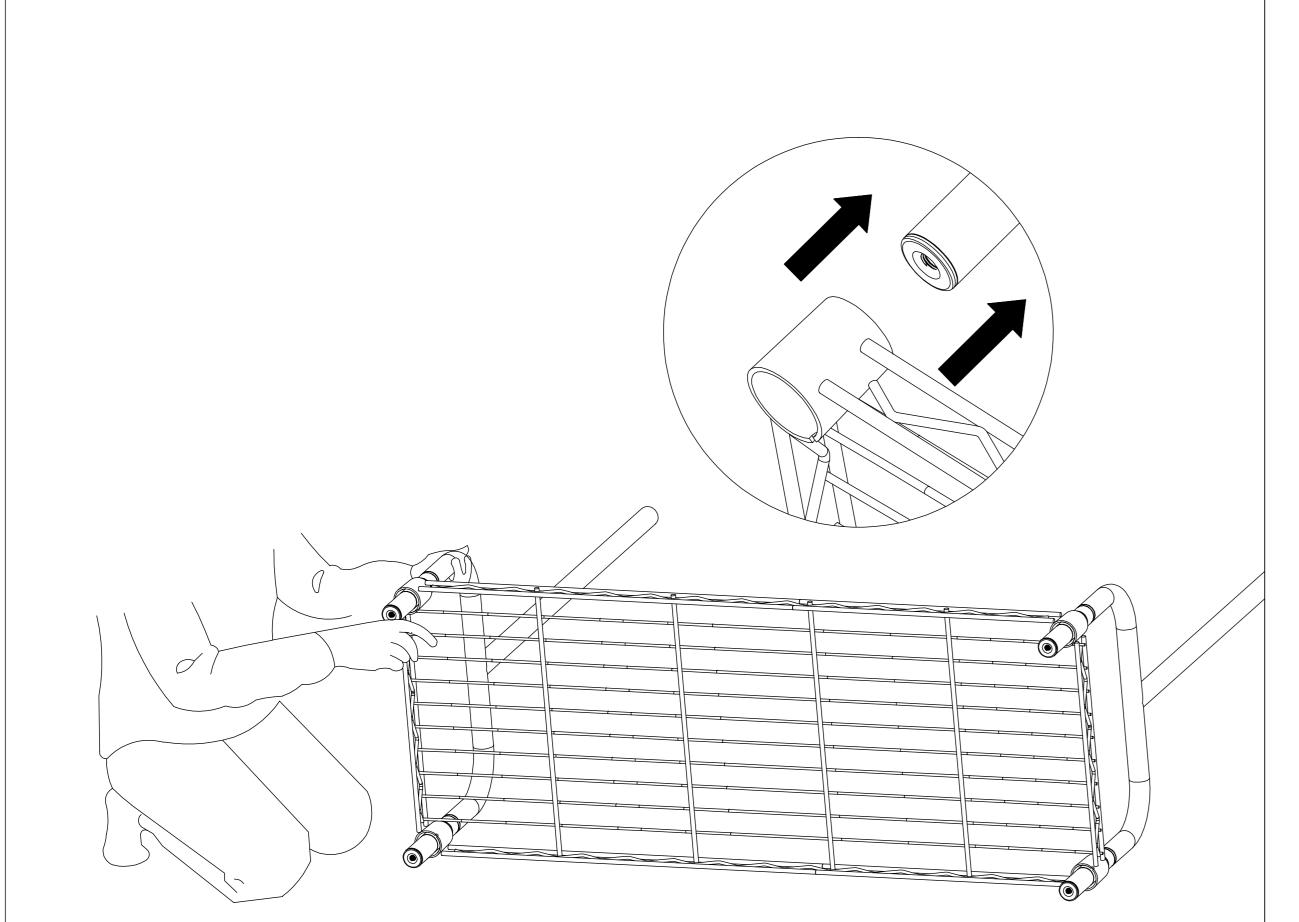
2 Snap the Plastic Clips(G) into the grooves of Y-shaped Poles at your desired position for the wire shelf,make sure that the plastic clips is under the wire shelf and it's arrow pointed up. Then press wire shelf firmly down onto the plastic clips.
