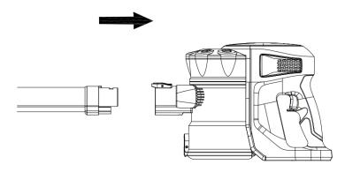
2. Attach the accessory to the base of the extension tube via the connector. It will "click" into place.
