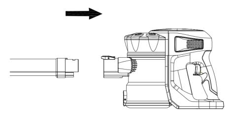
3. If using the motorized illuminated floor brush without the extension tube, simply attach it to the main body. It will "click" when secure.
