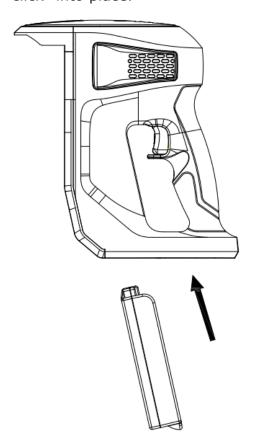
2. Install the dust container by inserting the clip into the main body, then put the upper side into place. It will "click" to secure.
