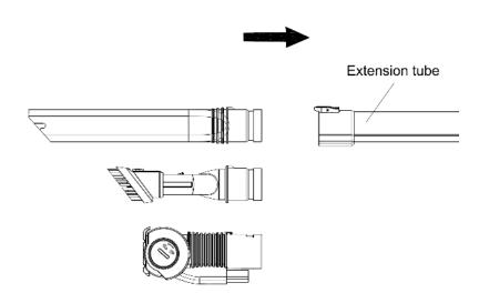
3. If using accessories without the extension tube, simply attach them to the main body. It will "click" when secure.
