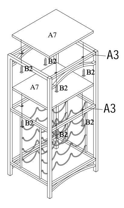
Attach Wood Panels (A7) to Side Frames (A1) and Connect Bar (A3). Then tighten all (B1) bolts and fasten with screws (B2).
