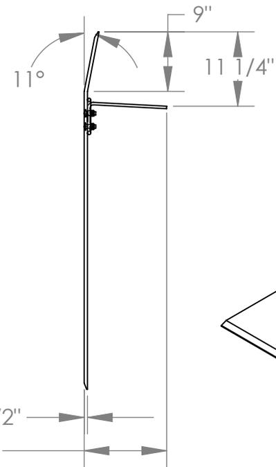
NOTE: BEND OR CROWN IS 11° AND LOCATED 9" FROM EDGE OF DOCKPLATE
