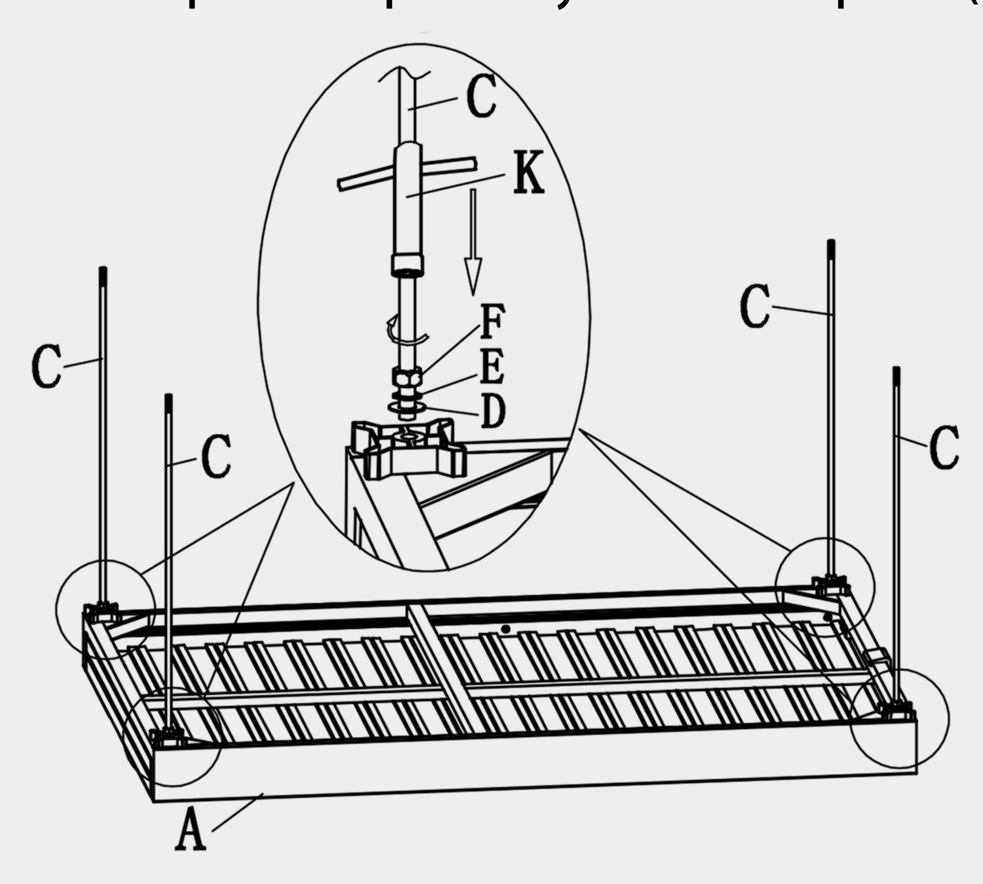
Step 2: Cover part C with part B, then put D,E shown in the diagram. Then lock part F(screw) using part K(Tool).
