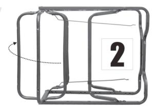
Cross bar must be positioned between caster and leg flat side facing up.
