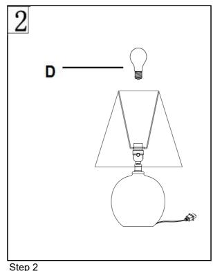
Insert the bulb(D) into the socket(B).
