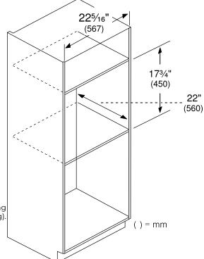
NOTICE: The cabinet base must be flat and capable of supporting a weight of at least 142 lbs (64.1 kg).
