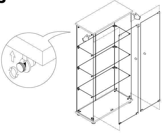
After installation, it must be anti-tipping device to a solid wall to prevent tipping and shaking!
