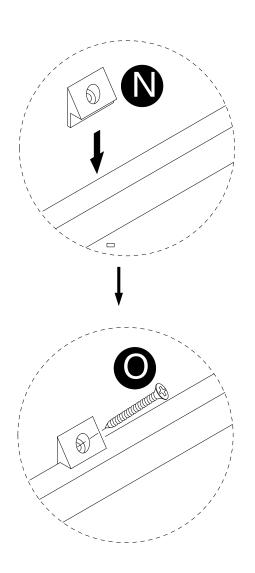
· Secure parts (N) to panel (15) with screws (O).
