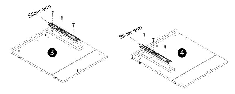
· Attach slider arms to panels (3,4) with screws (S) correctly.
