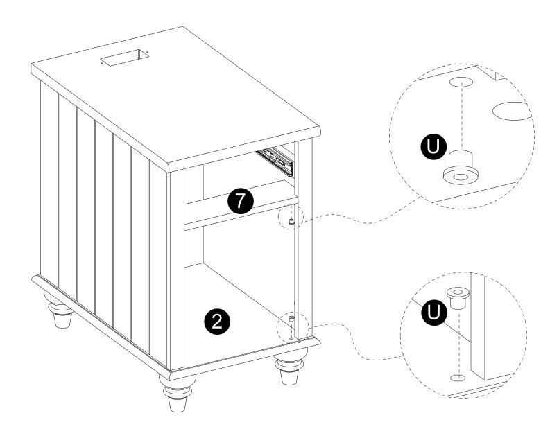
· Insert door shaft support (U) into panels (2,7).
