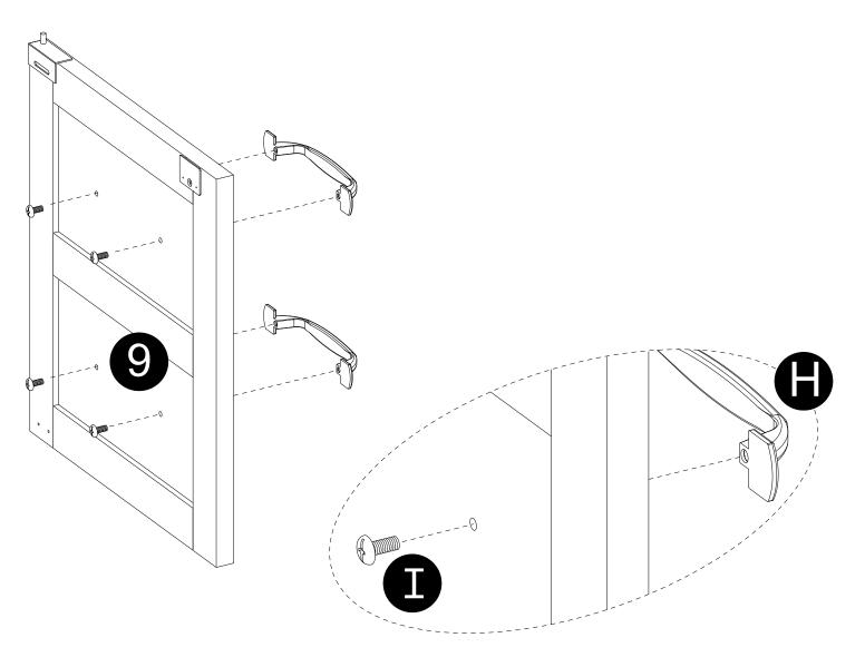
· Attach handles (H) to panel (9) with bolts (I) correctly.
