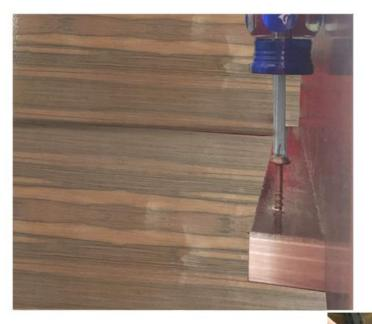
STEP 7: TAKE FOUR LONG SCREWS AND SECURE THEM WITH SCREWDRIVER IN THE FOUR CORNERS OF THE TOP PIECE AS SHOWN.
