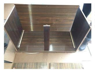
STEP 6: INSERT A DOWEL ON EACH END OF THE DIVIDER (PART C). SECURE IN FRONT OF TOP PIECE.
