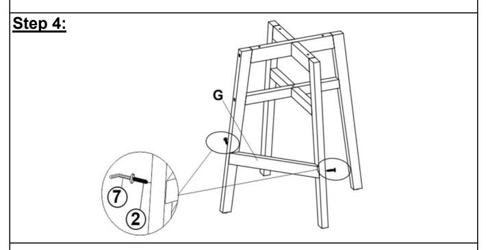
Secure the Footrest (G) to the assembled part of Step 3 using Screws ((2)) and the Allen Wrench ((7)) as shown in the picture above.
