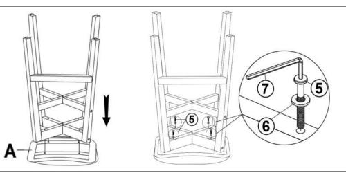
Place the Seat Panel (A) onto the surface facing downwards, as shown above. Insert the assembled frame of Step 4 to the Seat Panel (A) using Bolts (5) and Flat Washers (6) with the Allen Wrench (7) as pictured above.
