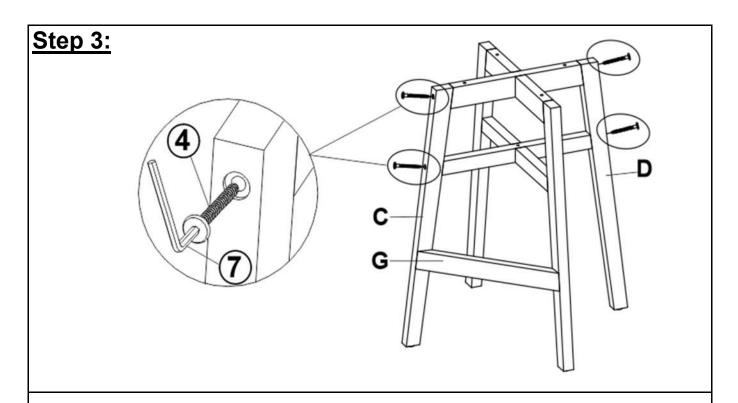
Attach the Second Leg (C), Third Leg (D), and Footrest (G) to the assembled part of Step 2, using Screws (4) and the Allen Wrench (7) as shown above. **DO NOT** fully tighten the Screws at this time.
