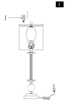
Step2 Insert the bulb(I) into the socket(E).
