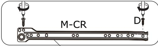
Fix slide rail(M-CR) and (M-DR) to No.11 and No.12 plate respectively using screw(D) as shown.
