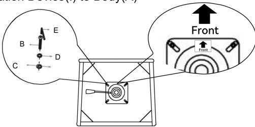
Step 3:Insert the wheels into the bottom of leg and the gas pole into the leg
