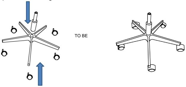
Step 4:Insert the leg into the Rotation Device under the
