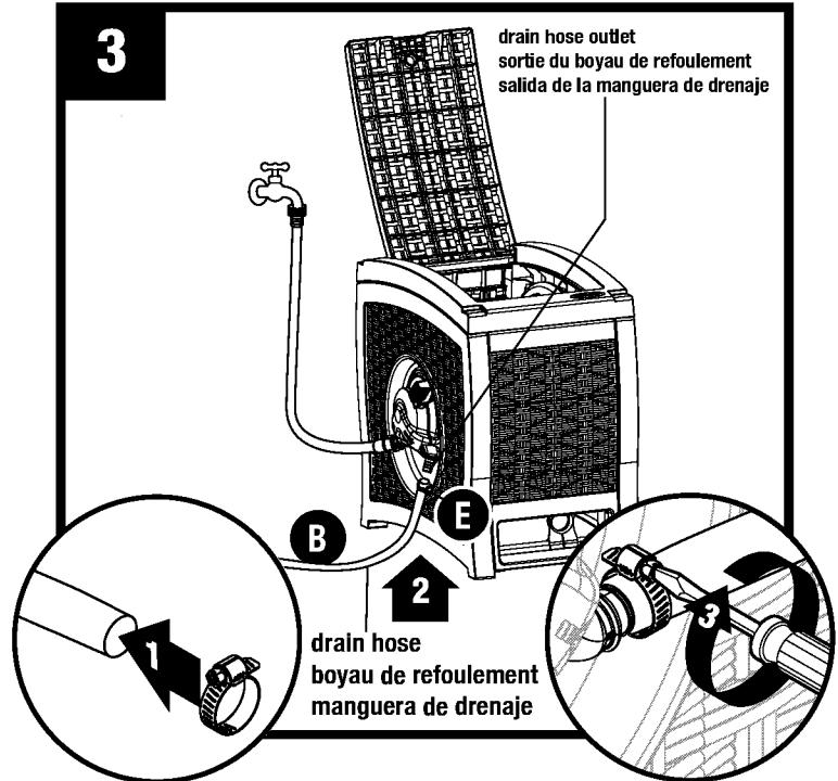
**Connect Drain Hose (B).** Attach hose clamp (E) to drain hose. Connect one end of drain hose to drain hose outlet. Tighten hose clamp with flat head screwdriver. Place the other end in a suitable water drainage area.
