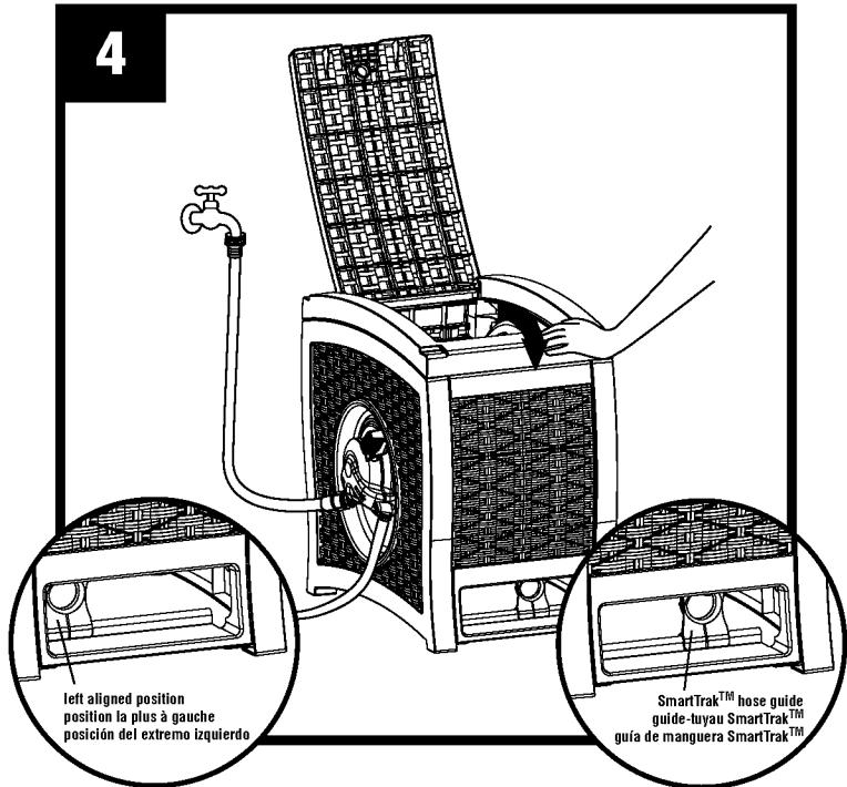
**Align SmartTrak™ Hose Guide.** Manually rotate drum until the hose guide is in the left most position.
