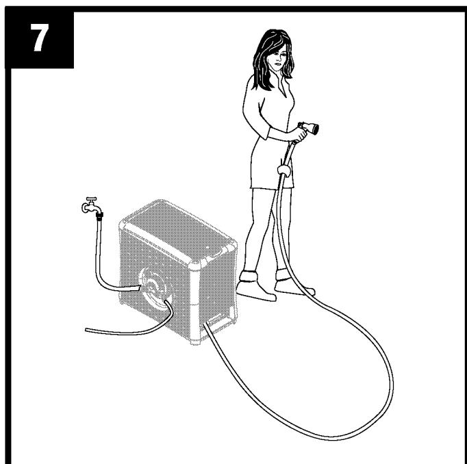
To wind your hose, pull the hose out away from your hose reel in a straight line. Then walk the end back to the hose reel so the hose is in a "U" shape in front of the reel. This assists in easier rewinding of the hose.
