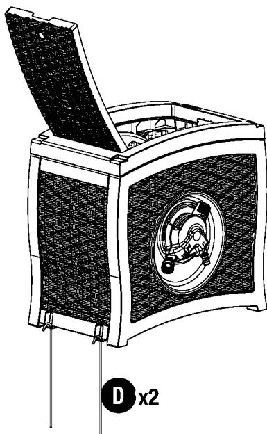
**NOTE: Stabilizing your hose reel by staking is recommended.**
