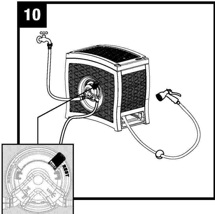
When finished rewinding garden hose, set the lever to REST and turn off the water source.
