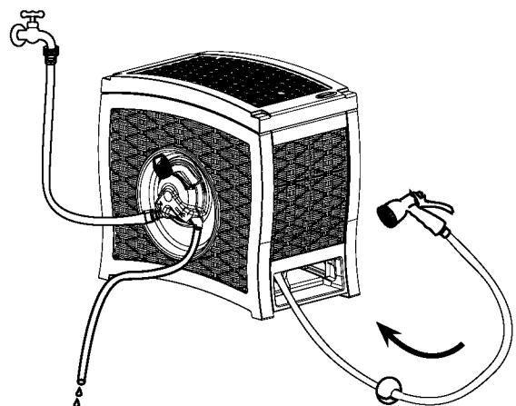
If necessary, guide your hose as it rewinds. The hose will stop rewinding when the hose stopper comes in contact with the unit.
