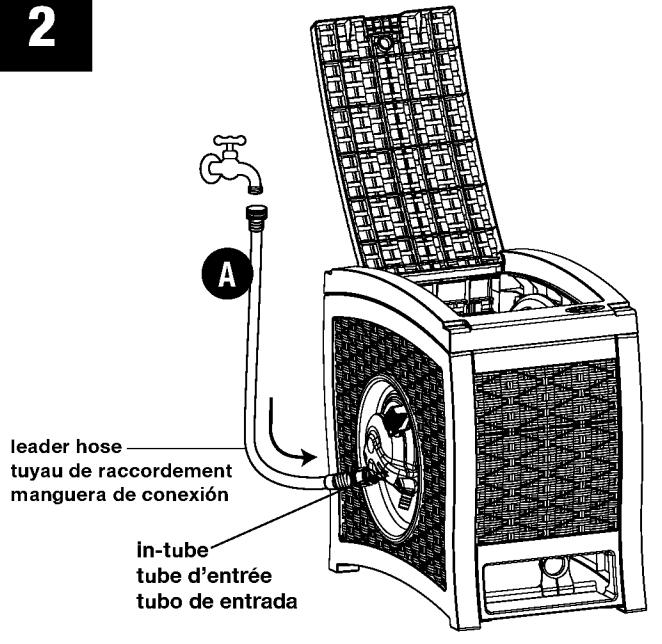
**Connect Leader Hose (A).** Thread male end of leader hose into in-tube. Thread female end of leader hose onto spigot.
