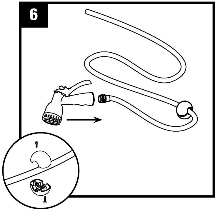
**Connect The Hose Stopper (C).** The hose stopper will stop the hose from rewinding when it comes in contact with the unit. Position the hose stopper near the end of the hose. Attach firmly with screws. Attach the hose nozzle (not included).
