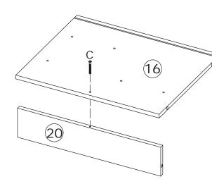
Fix board 19 to board 14; board 20 to board 15 and 16; board 21 to board 17 with screw(C) as shown.
