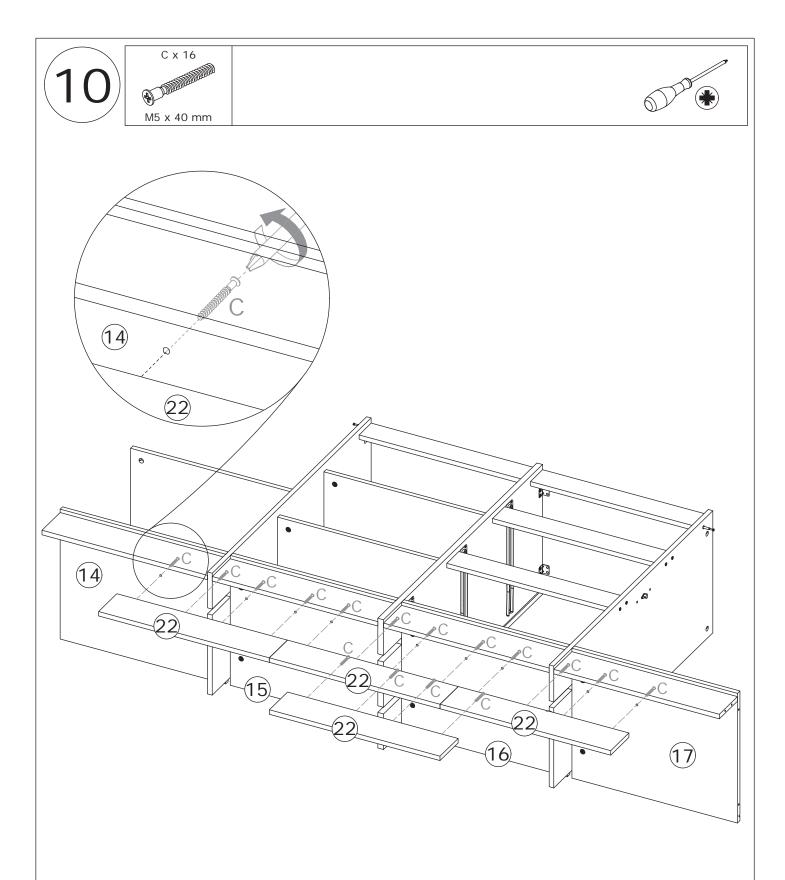
Fix board 22 to the unit with screw(C) as shown.
