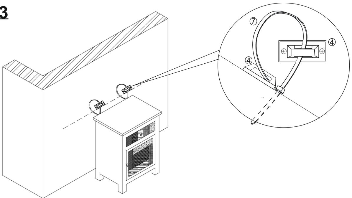
Move Bedside to the wall. Pull the Restraint Straps (7) through the Brackets (4) on the wall and Bedside one by one , and pull the Restraint Straps (7) tight.
