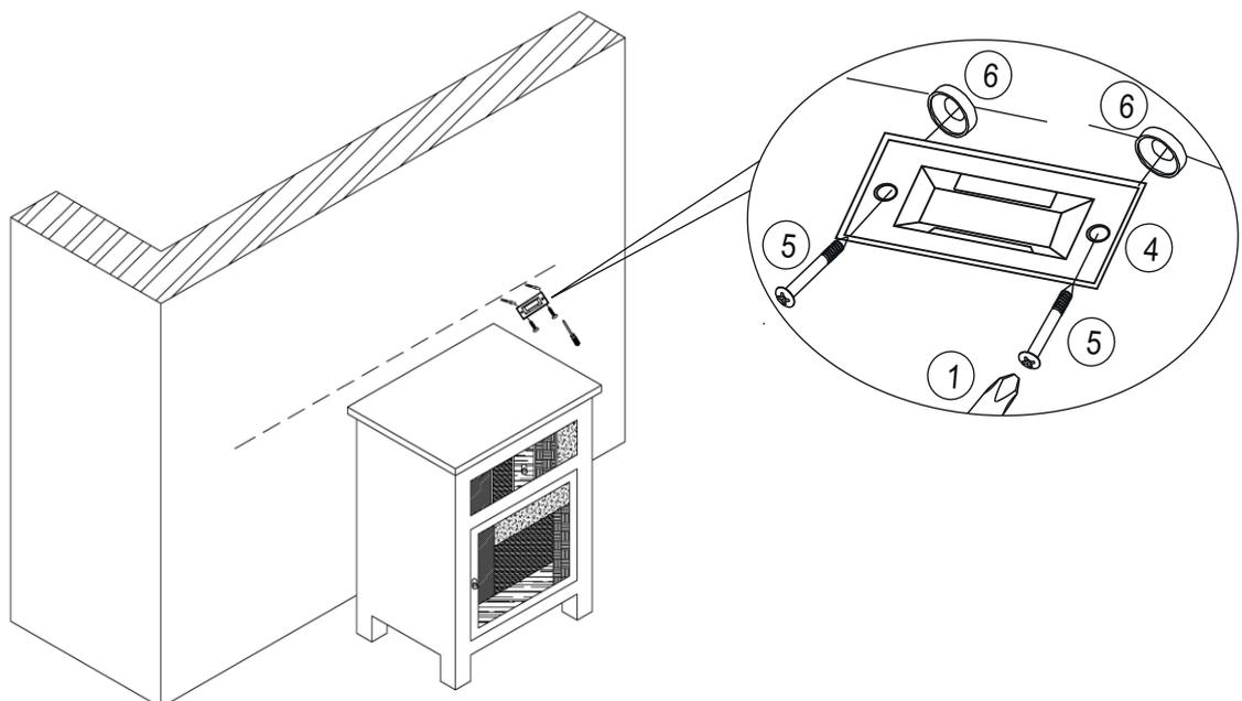
Attach Brackets (④) to Wall Plugs (⑥) using Wall Plug Screws (⑤) with Screwdrivers (①)
