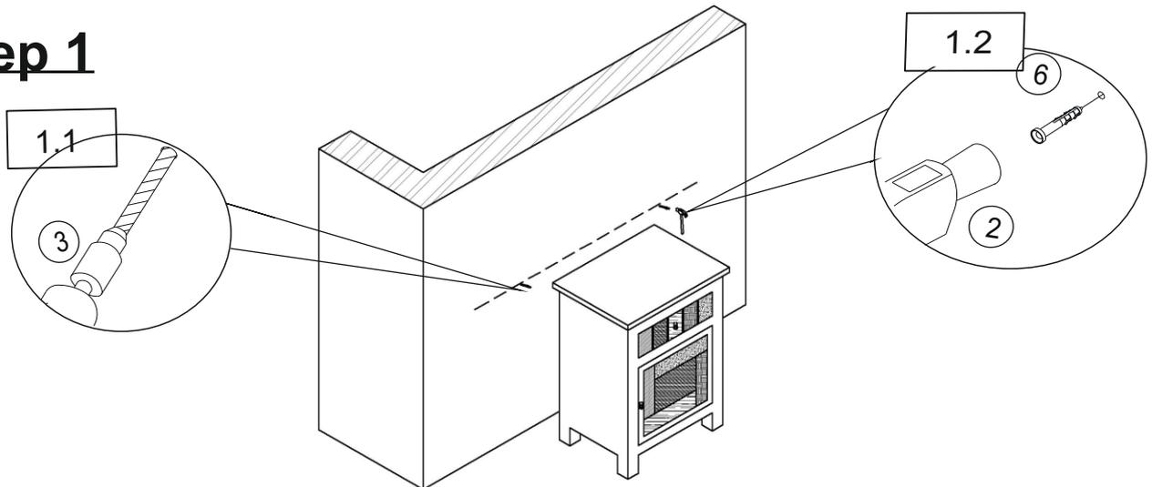
1.1) Drill two holes on wall at same height as Bracket (④) on Bedside with Power Drill (③).
