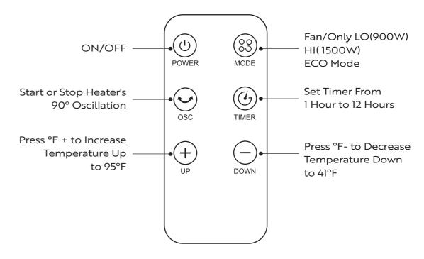
Note: Switch to ECO mode to adjust thermostat from 41°F to 95°F (in 1°F Increments)
