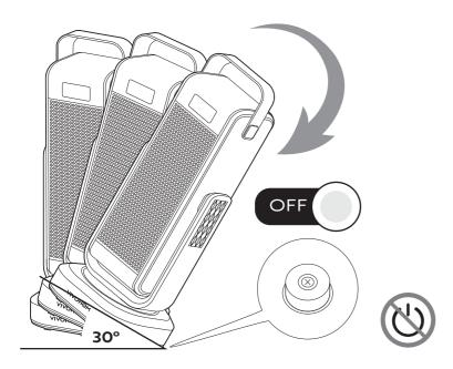
When the heater is tipped forward or backward, or knocked down by accident, the tip-over switch in the bottom will activate and shut off the heater automatically. So please put it on a flat surface to use the heater. Tips: After tipping over, if you want to continue using it, place it horizontally, then turn on the power switch and reset the mode you want.
