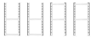
Step 3 : Setting Up the Beams and the Braces
