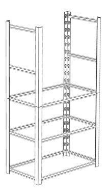
Please note that the middle layer needs to be connected with upper and bottom post to increase firmness, so it can not be adjusted up and down
