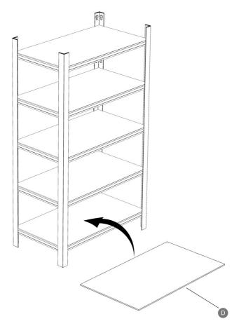
Hold the press board at an angle to make it easier to fit them onto eac previously assembled level on the frame.
