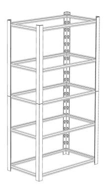
Repeat step 2 and step 3 to assemble the remaining beams and braces
