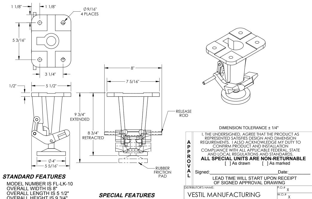
**OVERALL HEIGHT IS 9 3/4"** WHEN EXTENDED **MOUNTING HEIGHT IS 9 15/16" USED WITH CATER SIZE 8"**
