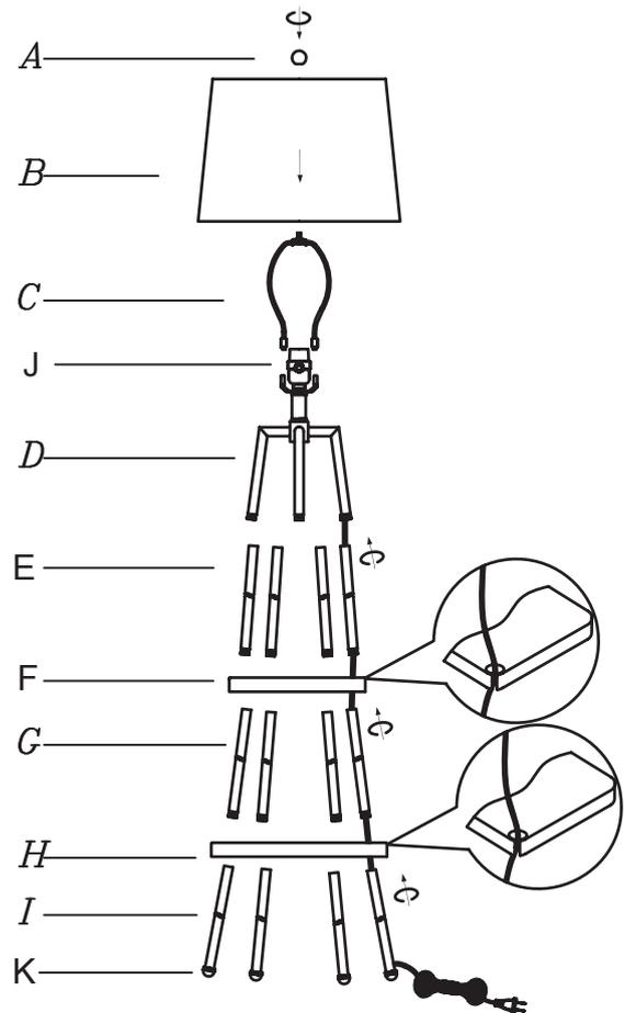
**NOTE:** If the floor is not flat, turn the adjustable foot pads (K) to stabilize the lamp.
