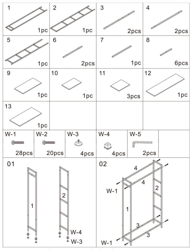
**Notes:** Don't tighten screws completely at first, just in case parts were assembled wrong and need disassembled. Tighten screws at last when all parts are put together.
