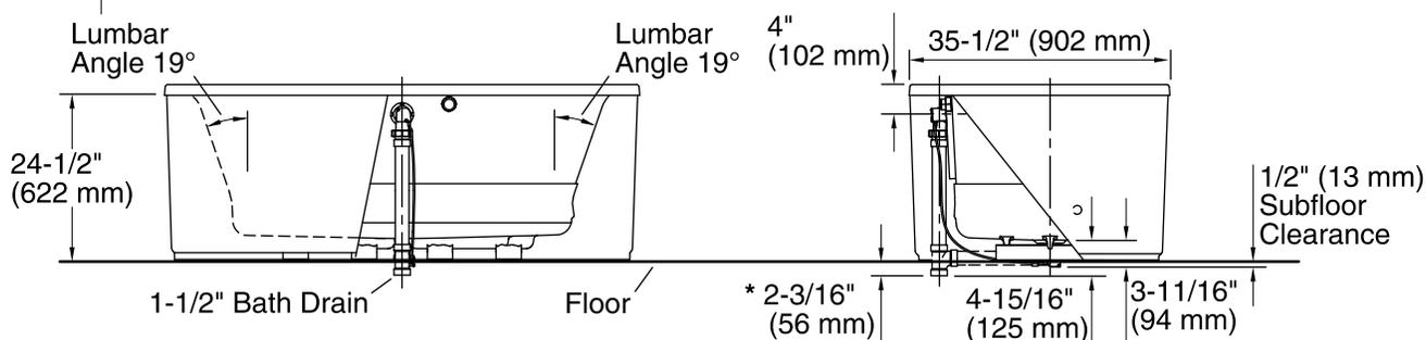
\* Allow for appropriate clearance in subfloor for drain clearance.
