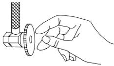
Locate water supply inlet and shut off water supply valve. Remove old handle trim. Clean and dry surface area where new handle trim will be mounted.
