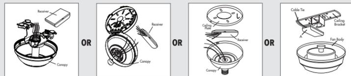
**Note:** Some fans may have considerable excess lead wire. For easier canopy installation, cut the excess wire, leaving a minimum of 8" remaining. Re-strip the fan lead wires 1/2". Place remaining excess wire into the ceiling electrical box. **The bracket and fan must remain properly grounded.**
