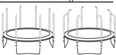
8. After connecting all enclosure poles insert the pole caps, if you have an inside type net use part number E1 and for outside type Net use E2. If you are using the curved poles, use the pole caps provided.
