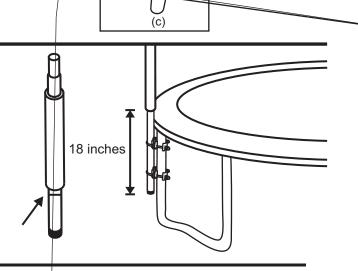
4. The set comes with 2 clamps per pole. One being attached 2" **below frame**, while the other being attached 2" **above the end of the lower pole**.
