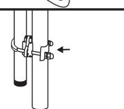
6. Now you can have the upper part of the pole inserted into the lower part that is already attached to the leg.
