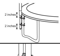
5. Insert the plastic bracket, then clasp the trampoline leg into the clamp. Secure tightly with steel brackets and nuts.
