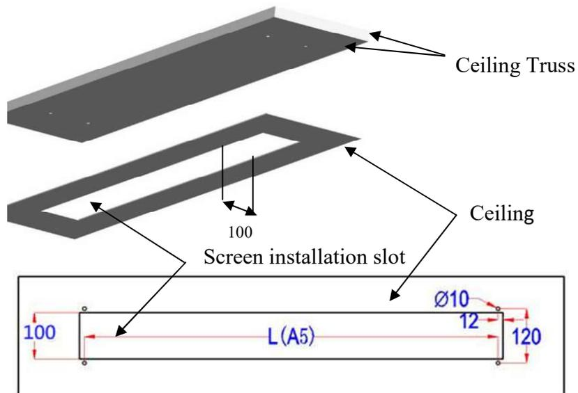
2. Drill 4 holes in the ceiling that correspond with the attachments on the various casing sizes. The width should be 120mm. The length of (A5) in the diagram below depicts the distance between the holes located on each ear end of the screen's case.
