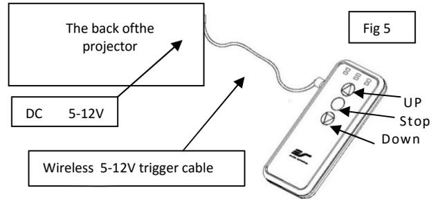
**Here's how to set up your Wireless 5-12 volt trigger | Synchronization Instructions**
