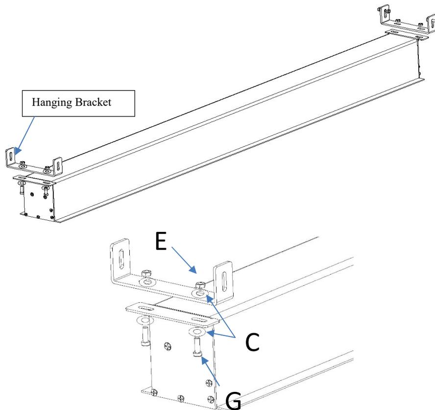
2. Place the **Suspension Bar (B)** over the **Hanging Bracket (A)** and align with the hole as shown below according to the height requirement for your installation area. Secure the **Suspension Bar (B)** with the **M6x20mm Screw (B)**, **M6x13mmx2mm Washer (E)** and the **M6 Nut (F)**. Repeat the process for the other side.
