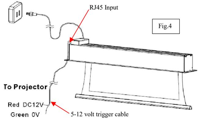
**6. Wireless 5-12 volt trigger (Item F, Fig 5):** The RF remote control serves as a dual purpose, independently as a handheld remote control, or in conjunction with the Wireless 5-12 volt trigger cable. The radio frequency technology can be programmed to send a wireless signal to synchronize its drop/rise with the projector's power cycle.
