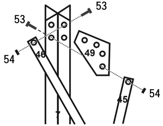
9. Insert a Brace Bolt (53) through the second hole from the top of the Corner Post (7) over the Front Floor Plate (1a). Place the bottom hole of the Corner Bracket (49) over the Bolt with it angled up towards the center of the greenhouse, as shown above. Secure it using a Nut (54).
