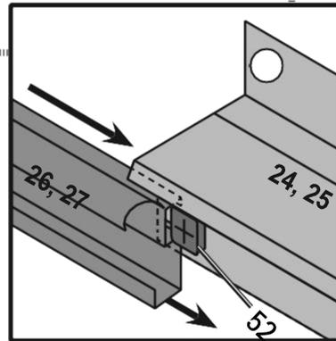
4. Slide the slot on the Left Door Rail (26) over the heads of the remaining three Bolts in the Front-left Ceiling Plate (24) until it presses against the Right Door Rail (27). Tighten the remaining Nuts.
