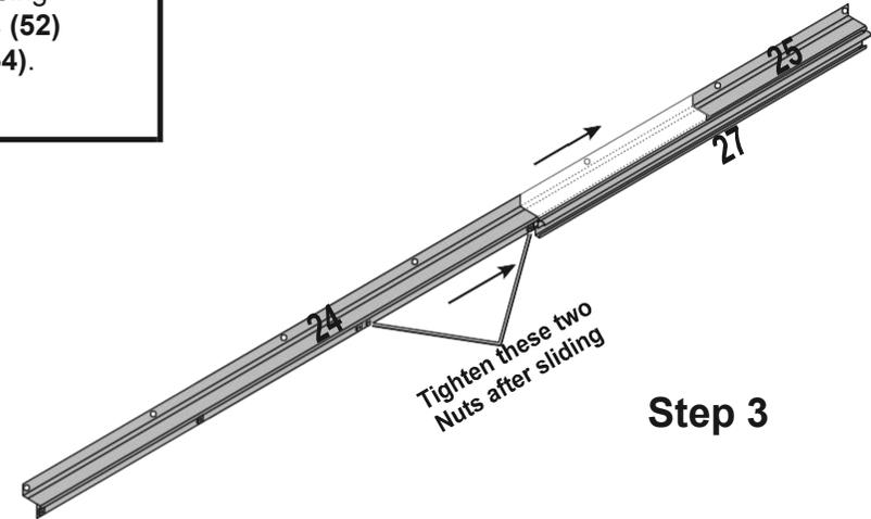
2. Slide the slot on the Right Door Rail (27) over the heads of the 2 Bolts on the Front-right Ceiling Plate (25) until the right end is flush, as shown. The illustration in the center of this page shows how to slide the Rail over the Bolt heads. Tighten the Nuts on those 2 Bolts.
