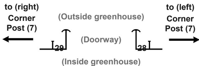
1. Using a Normal Bolt (52) at top and the Brace Bolt (53) already in place at the bottom for each, attach the Left and Right Doorway Posts (28, 29) to the outside of the Front Floor Plates (1a, 2a) and to the inside of the Front Ceiling Plates (24, 25). Install the Posts with the cut-outs at top and oriented as shown in the illustration above.
