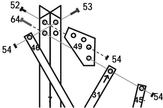
3. Fasten a Corner Bracket (49) to the top of the Corner Post (7) over the Rear Floor Plate (6) using one Normal Bolt (52) for now. Install it angled up towards the center of the greenhouse, as shown above.
