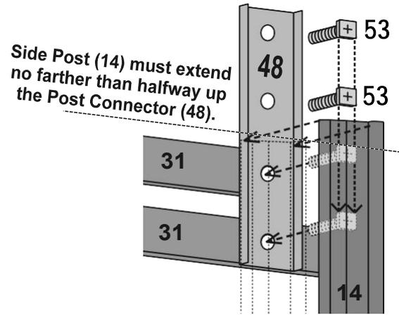
7. Remove the two Brace Bolts (53) connecting the Post Connector (48) near that Side Post. Slide the heads of those Bolts into the Side Post and insert them through the Post Connector. Align the top of the Post with the **center** of the Connector as shown above, and press it in place. Reattach the Rear Braces (31) to the Brace Bolts (53) and secure them.
