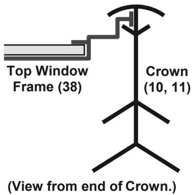
5. Hold the assembled window level with the ground at the outer edge of the Crown (10, 11). Slide the top edge of the Top Window Frame (38) into the slot at the top of the Crown – see illustration to the left. Align the window with the bottom Window frame(40) underneath it. Gradually lower it into place.
