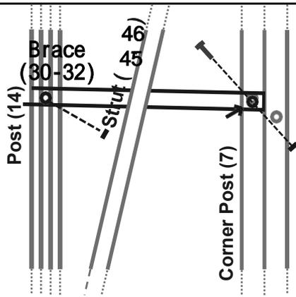
**Note:** All Braces are installed inside the Posts, but outside the Struts. See diagram above, shown from inside the greenhouse facing out.
