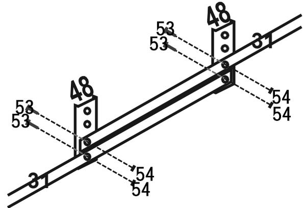
6. Bolt two Post Connectors (48) to a Rear Brace (31) using Brace Bolts (53) through their bottom holes, from the outside in. Place Post Connectors on the outside of the greenhouse with the flat side against the Brace, as shown above. Only finger tighten for now.
