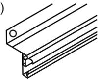
5. Attach the remaining Side Ceiling Plate (12, 13) along the other side according to steps 2 & 3, with the gutter opening up.
