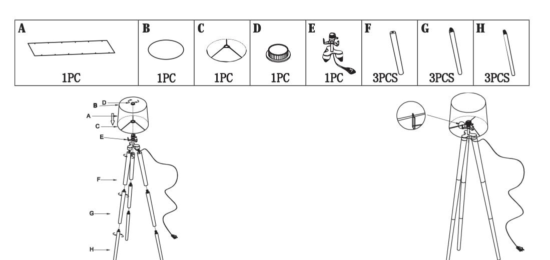
1. Screw the leg parts into one another. Place the shade on the lamp body. Secure the lamp shade with ring (D). See separate shade assembly instructions.
